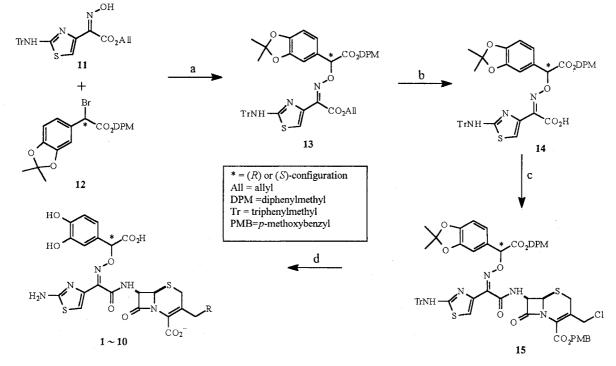
a) K<sub>2</sub>CO<sub>3</sub>, KI, DMF; b) Pd(PPh<sub>3</sub>)<sub>4</sub>, potassium 2-ethylhexanoate; c) POCl<sub>3</sub>, 7-ACLE; d) (1)Nucleophile (R); (2) TFA, Anisole.
